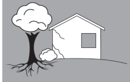
Damage from nearby tree
